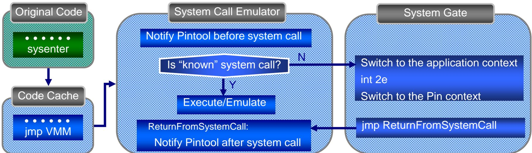
System Gate executes system calls “blindly”, assuming that each of them can arbitrarily modify context and control flow (if interrupted)
